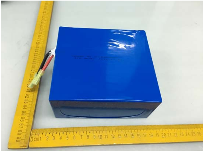
电池/ Battery(18650-16S3P 59,2V 6300mAh 372.96Wh)
